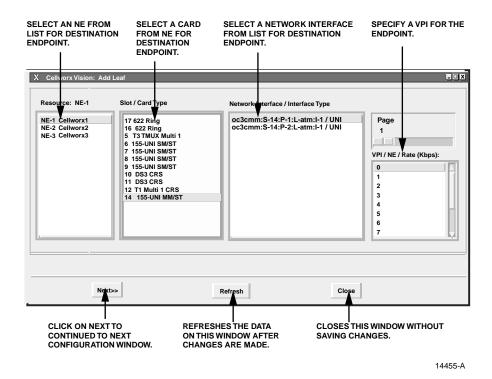
Figure 791-6. Add Leaf Window - NE, Slot, VPI Selection
